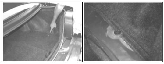
**STEP 2:** Remove the rubber plug, exposing the hole in the floor of the trunk.
